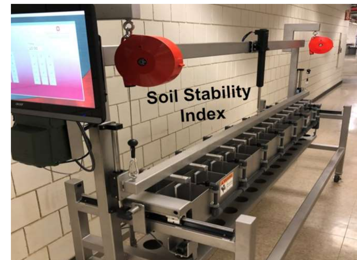
Combination of wet and dry sieving at multiple sieve sizes (Franzluebbers et al., 2000)
