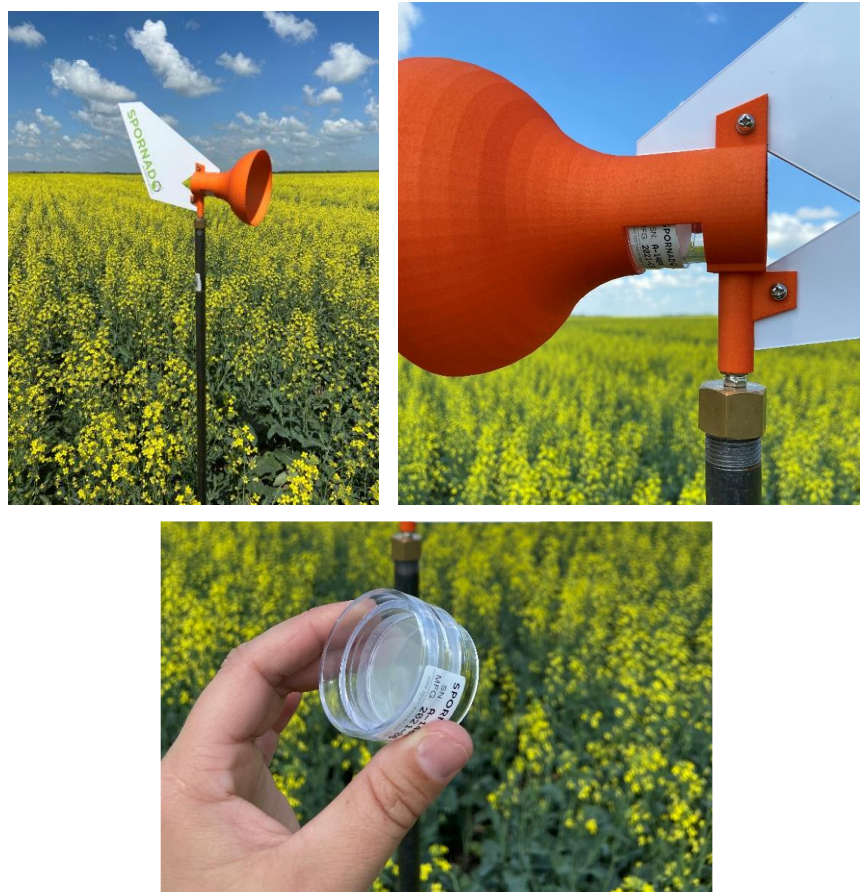
Figure 1. Spornado spore sampler installation and cassette insertion.
