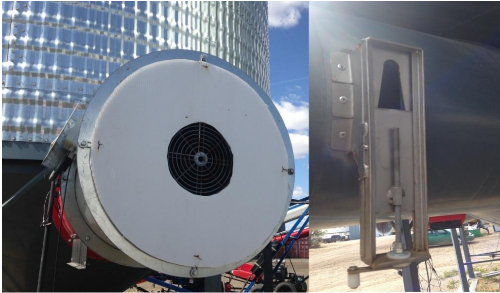
Figure 3: Inlet reduction cover and air vent to reduce cfm/bu.
