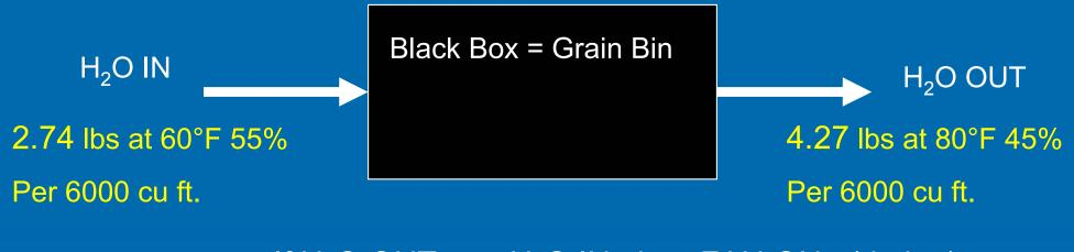
If  $H_2OOUT > H_2OIN$  then FAN ON (drying)
