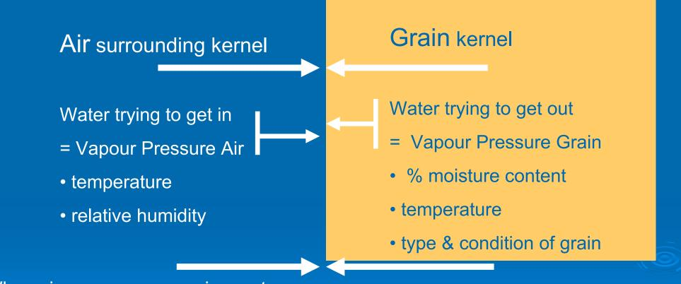
When air vapour pressure is greater than grain vapour pressure, water enters the grain and WETTING occurs. When Vps are equal,  $\rightarrow$  EMC
