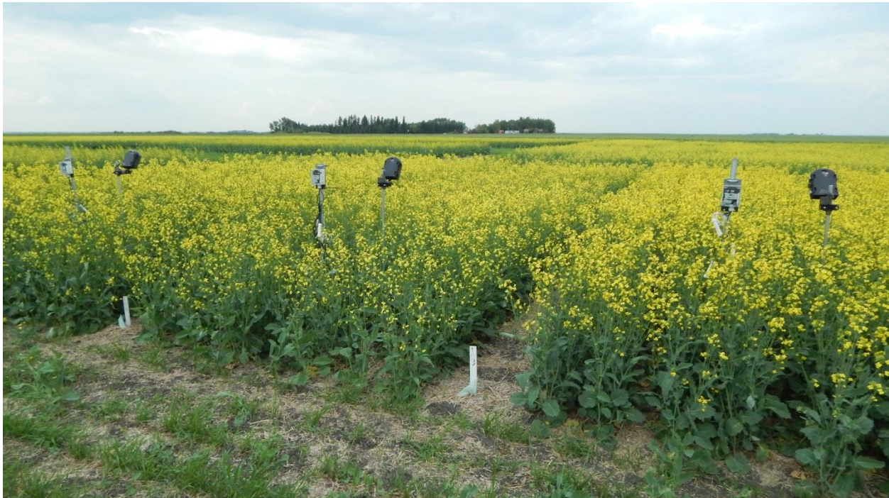
Figure 21. Photograph showing fixed time-lapse cameras and micro-weather stations installed in plots of canola with differing maturity ratings.
