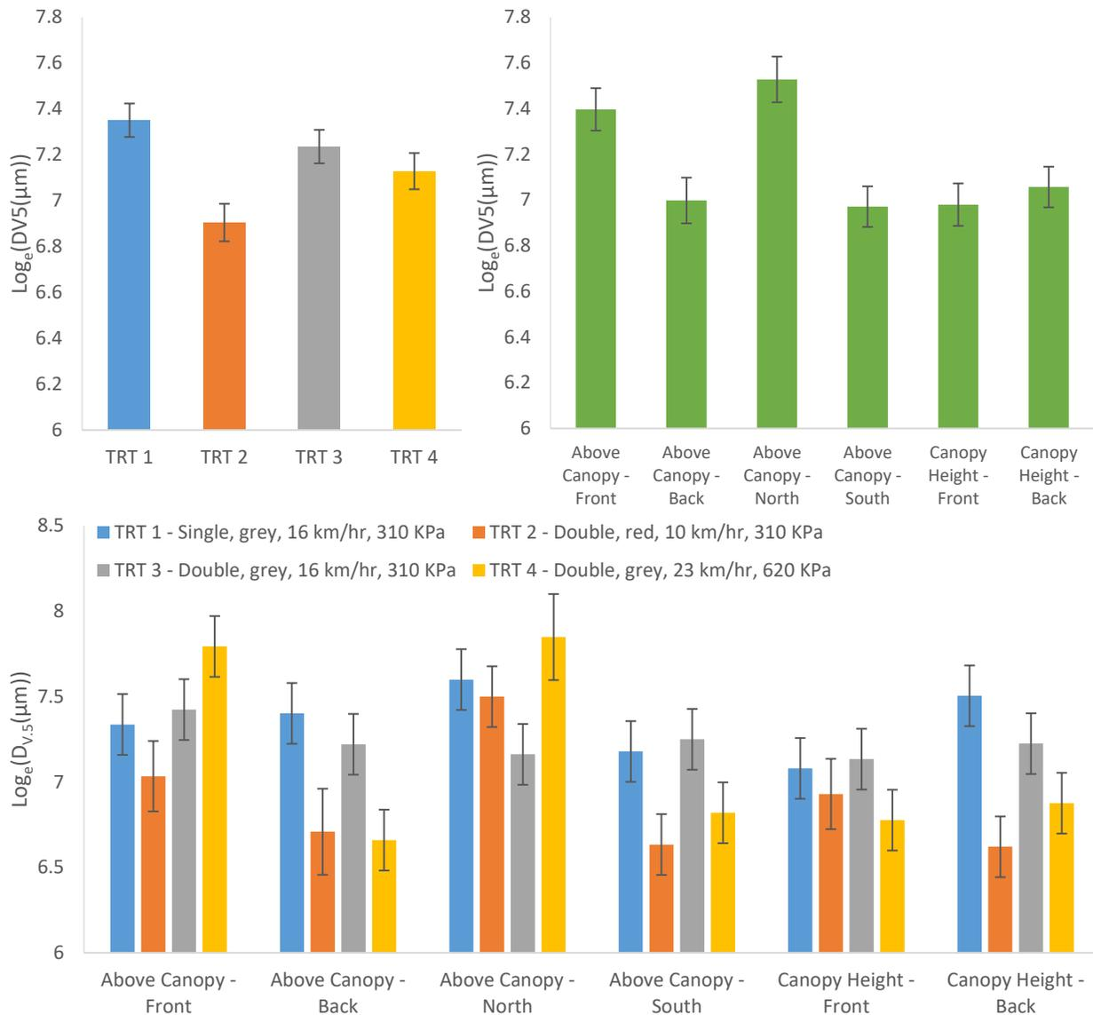
**Figure 1. Least squares means for the effect of treatment and location/direction of water sensitive paper on droplet size. Error bars indicate the standard error. Log-transformed data is shown so that the standard errors can be used to compare treatment effects.**
