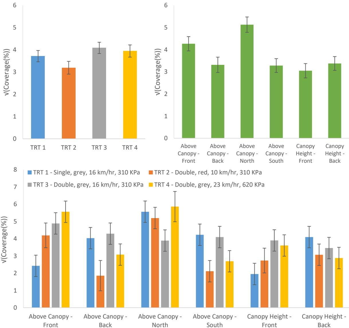
**Figure 2. Least squares means for the effect of treatment and location/direction of water sensitive paper on percent coverage. Error bars indicate the standard error. Square root-transformed data is shown so that the standard errors can be used to compare treatment effects.**
