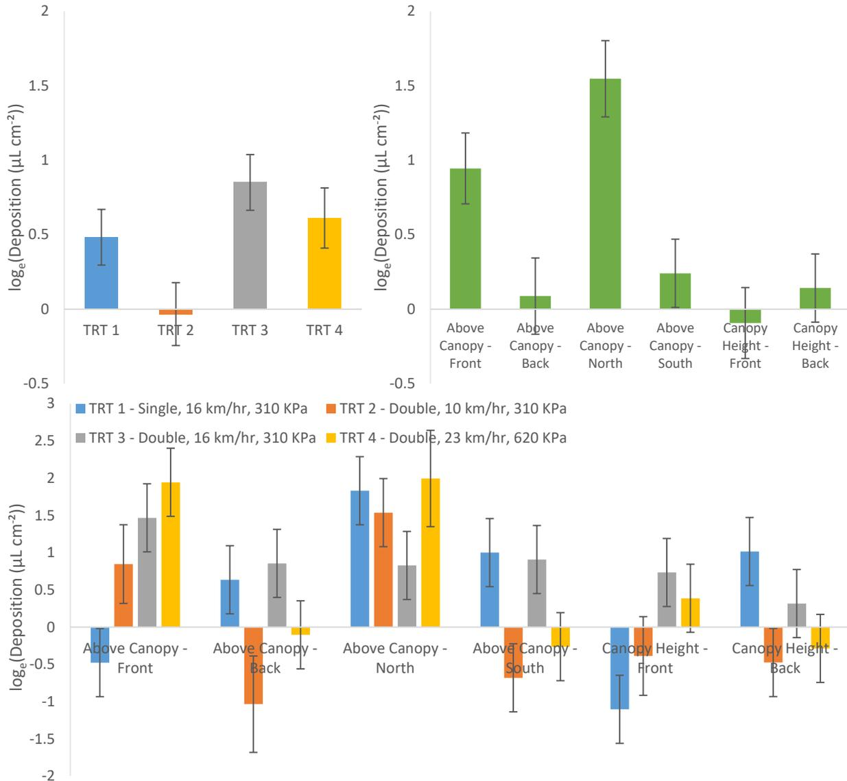
**Figure 4. Least squares means for the effect of treatment and location/direction of water sensitive paper on deposition volume ( $\mu\text{L cm}^{-2}$ ). Error bars indicate the standard error. Log-transformed data is shown so that the standard errors can be used to compare treatment effects.**
