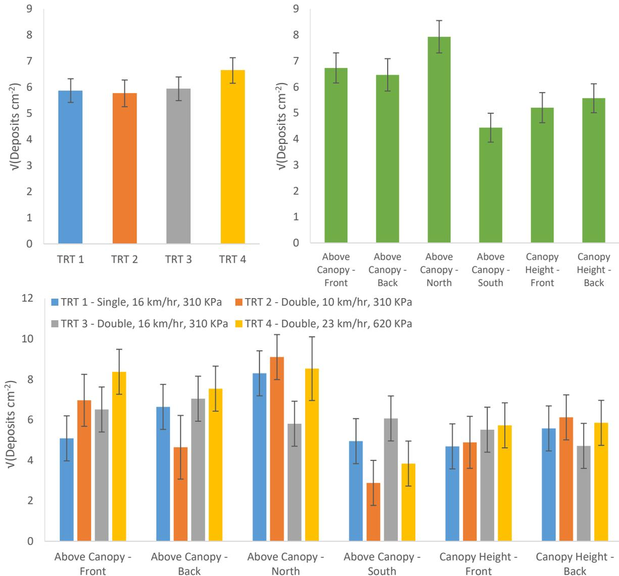
**Figure 3. Least squares means for the effect of treatment and location/direction of water sensitive paper on deposits  $\text{cm}^{-2}$ . Error bars indicate the standard error. Square root-transformed data is shown so that the standard errors can be used to compare treatment effects.**
