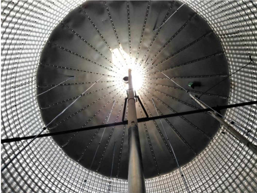
Figure 1: Sampling tube and sensor strings inside of test bin.
